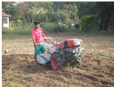
Ivan using our new rotor-tiller preparing the ground for sowing at "El Camino"
